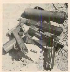
5. Withdraw bolt group from rear of 6: M10, field-stripped, including magazine and sound-suppressor.
